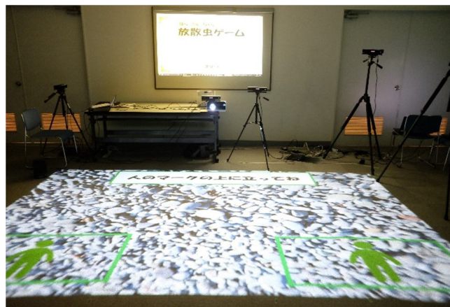
Figure 4: Link of two projectors. Depending on the learner's movements, the images and animations of the two projectors change.
